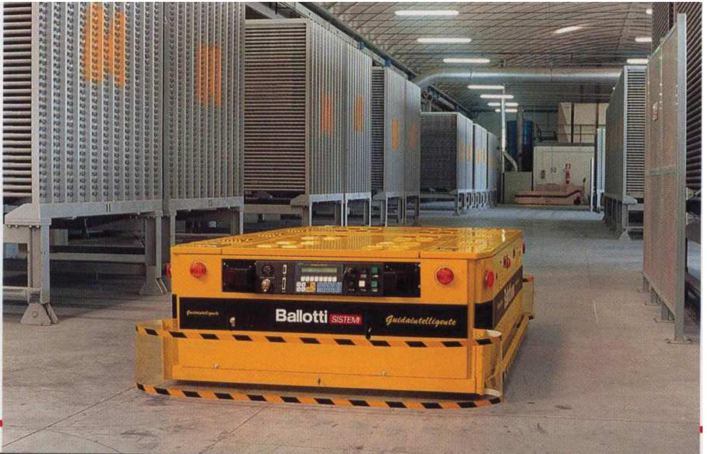
Example last model of AGV "turtle" with laser scanner
